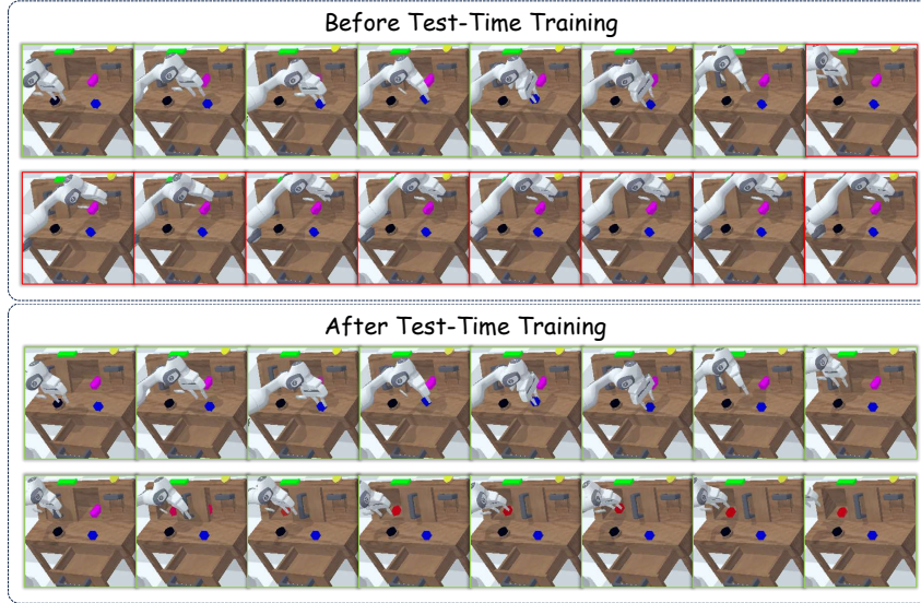
Figure 5 | In the comparison between the trajectories before and after TTT, the red regions indicate failures within the trajectory, while the green regions represent successful portions.
